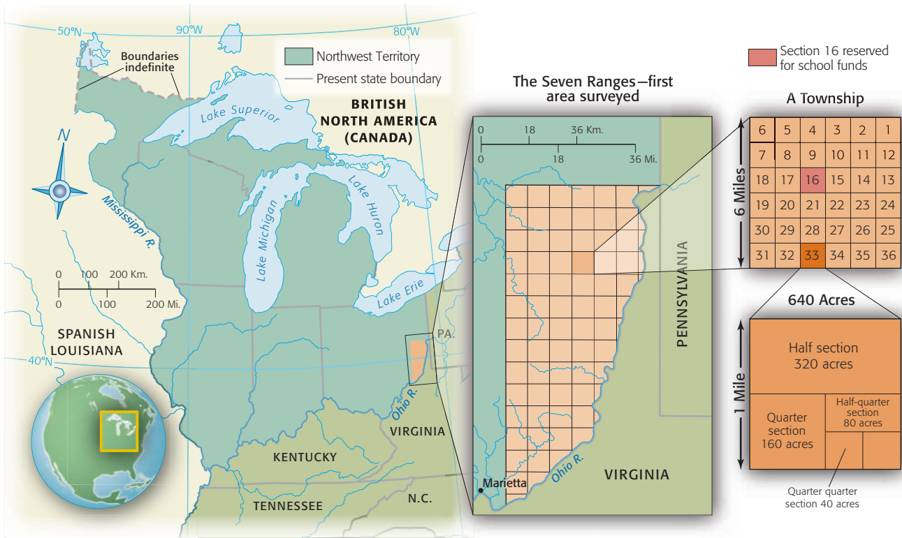
Map 9.2 Surveying the Old Northwest under the Land Ordinance of 1785 Sections of a township under the Land Ordinance of 1785.
